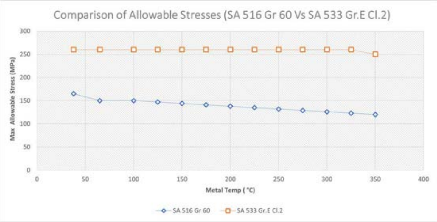
Figure - 1 : Comparison of allowable stresses for SA 516 Gr 60 & SA 533 Gr.E Cl.2
