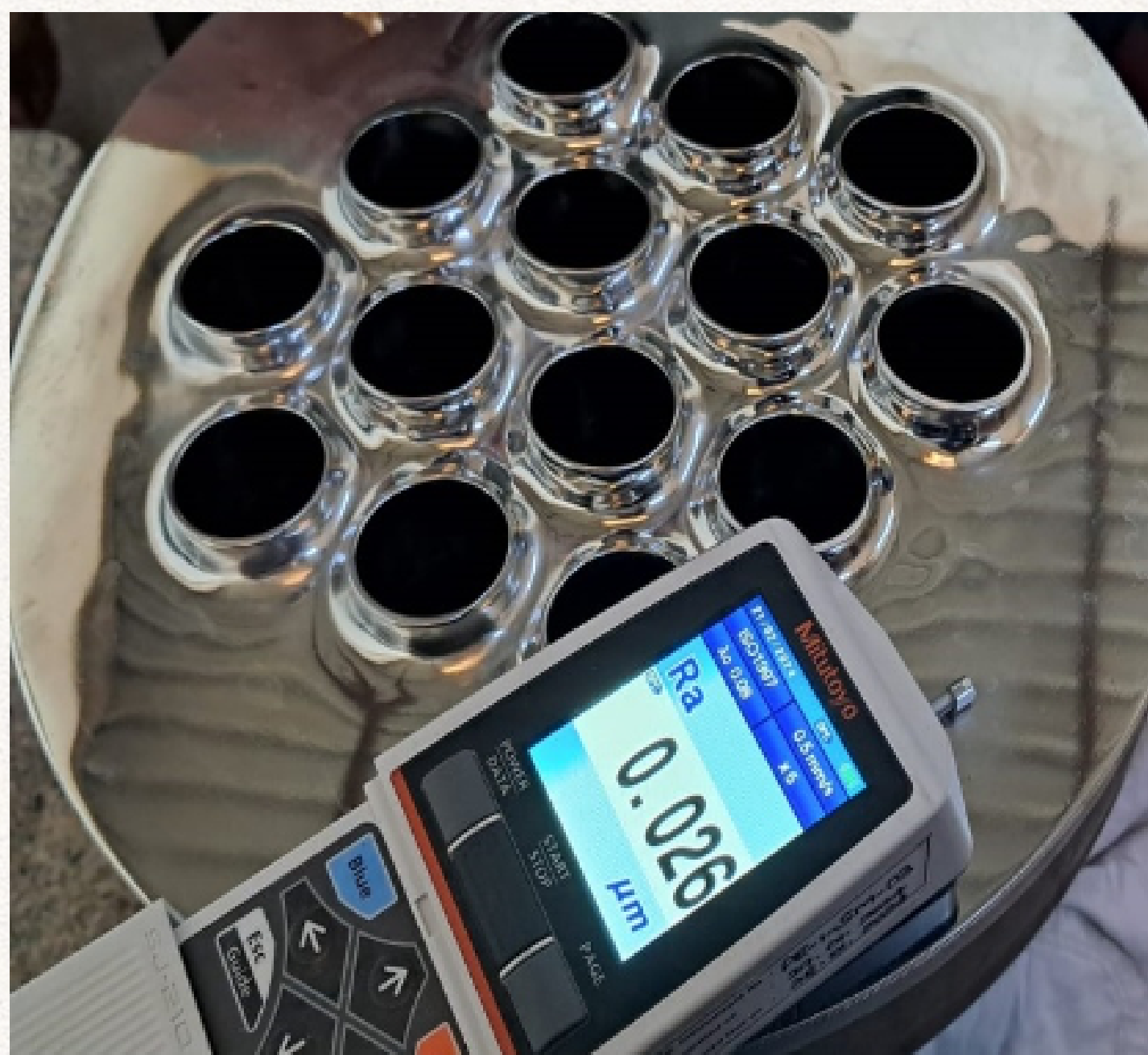
Fig 6. The surface roughness of mock-up is 0.026 is achieved after electropolishing.
